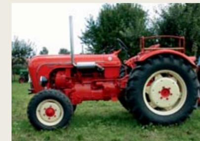
**Engine:** Four-cylinder with 3,288 to 3,500 cc
