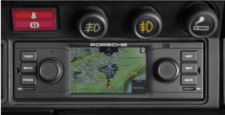
Operated via either the 3.5-inch touchscreen or the switches and buttons
