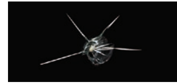
Star crack up to 40 mm in diameter
