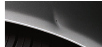
Dents in side wheel arch
