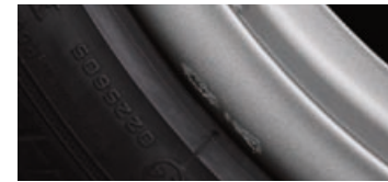
Alloy wheel with minor damage
