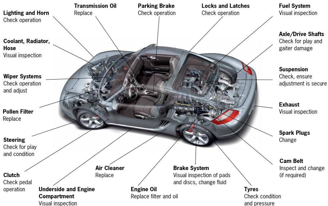
Service includes adjusting, readjusting, correcting and topping up of discussed components
